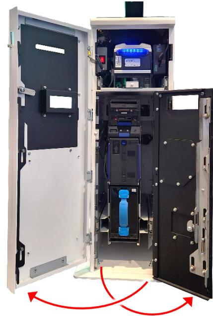
4. Remove the Stacker by simply pulling it straight out by the handle.
