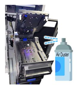
4. Use the Microfiber cloth to gently wipe the sensors and rollers clean. Do not use too much pressure and be careful not to damage or scratch the sensors.
