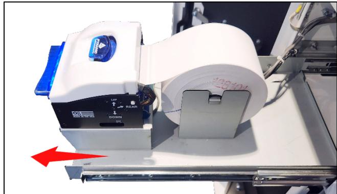
2. On the Left side of the Printer, check to be sure the Printer Power Cable is connected properly.
