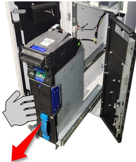
2. Press Down on the release latch on the front of the Bill Validator.
