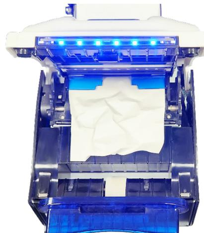
2. Unjam any damaged paper and pull the paper forward until clean, undamaged paper appears.
