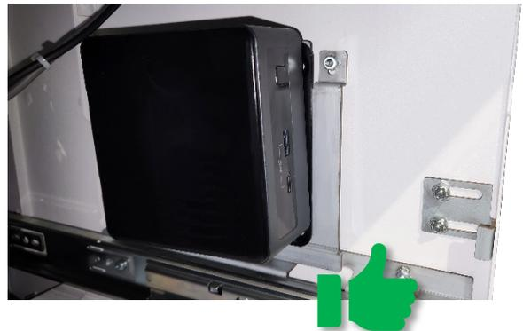
3. Lift and remove the Bac Mini PC from the Bracket.
