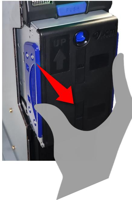
4. Insert the New Recycler and push in till it locks in place.
