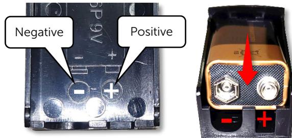
4. Return the Battery Housing to the Keypad.
