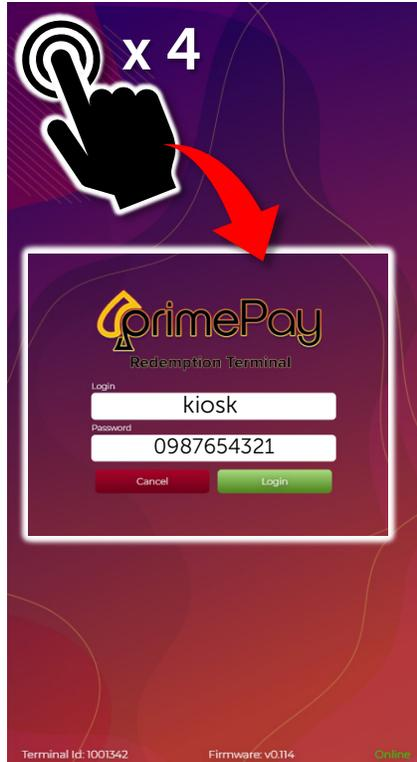
Tap the Upper Left corner of the screen 4 times to open the Operator Login.
