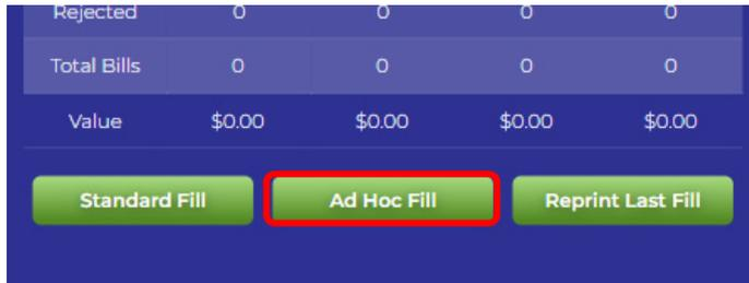
An Ad Hoc Fill allows the Operator to add a custom number of bills to a Cassette during a Fill. Unlike the Standard Fill which sets a specific number of bills to add to reach a set Fill Target, the Ad Hoc Fill allows the Operator to Manually Enter the number of bills being added to the Cassette.
