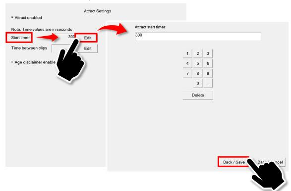
35. If desired, Tap **Edit** next to the Time between clips to change the duration between the Attract clips. Enter a New Value and Tap **Back / Save** when finished
