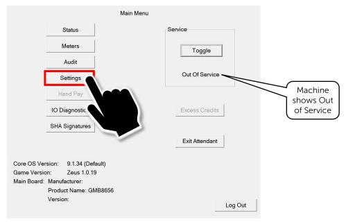
**Note:** Tapping the **Toggle** Button here will not put the machine in service. A Game must first be activated, or an error will occur.
