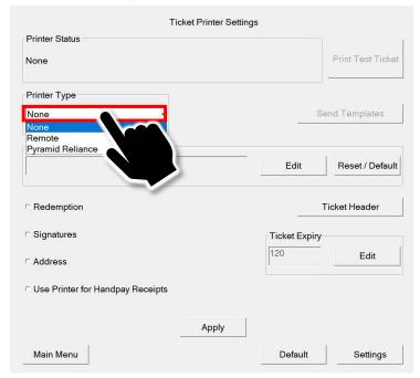
46. Once a new printer type is selected, the Printer Status will read: The printer type has changed, please press Apply.
