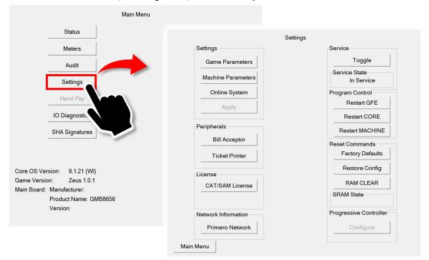
2. On the Settings screen, Tap Restore Config and the Restore Config Screen opens.
