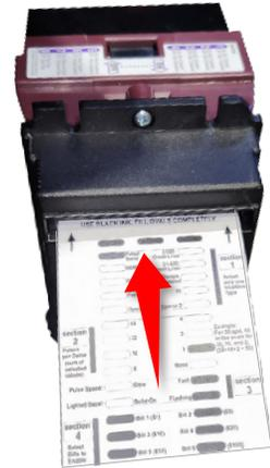
6. The bezel lights should flash rapidly, indicating the validator has read the Configuration Card correctly. The configuration is now in permanent memory in the Bill Acceptor which should now reset itself by doing a stacker cycle.
